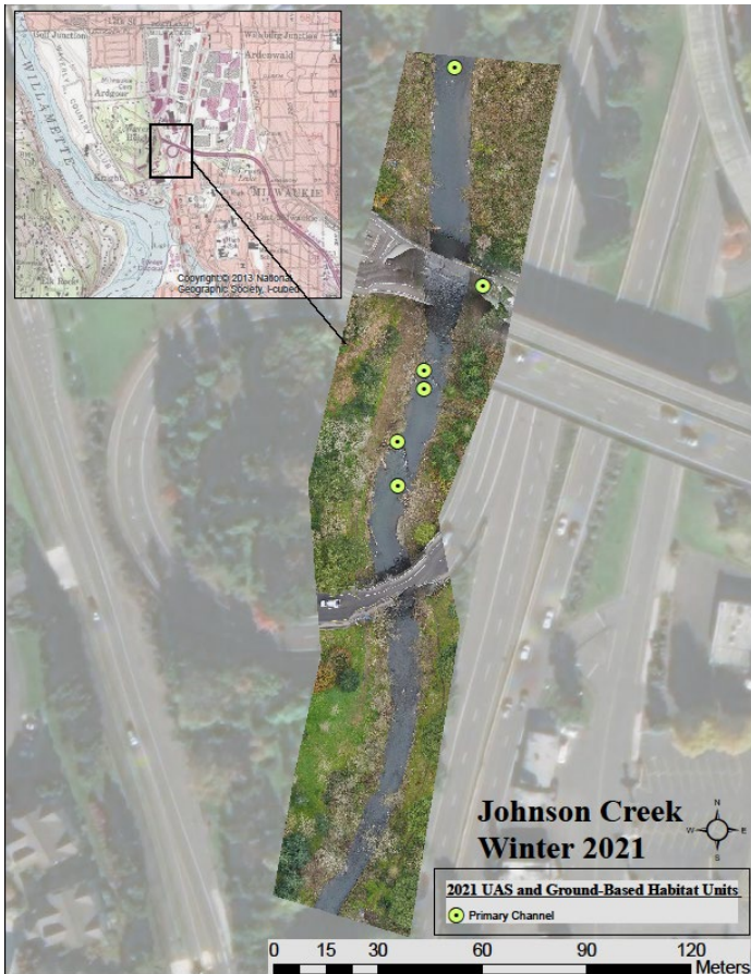
Figure 14. Johnson Creek. Winter 2021 UAS imagery and ground-based survey points.
