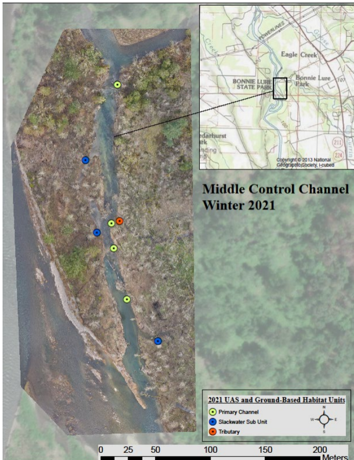
Figure 8. Middle Control Channel. Winter 2021 UAS imagery and ground-based survey points.
