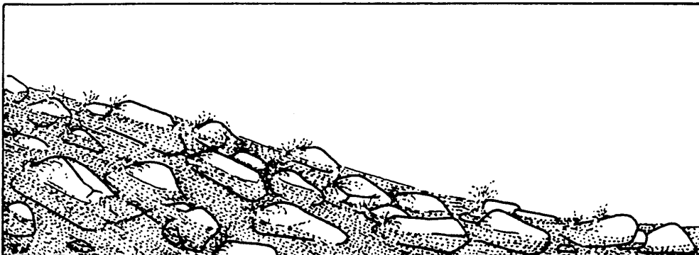
RB Rapid With Protruding Boulders: Swift, turbulent flow with chutes and hydraulic jumps, moderate gradient; usually 2.0 - 4.0 % slope, occasionally 7.0 - 8.0 %, 15 - 50 % of surface area with white water.
