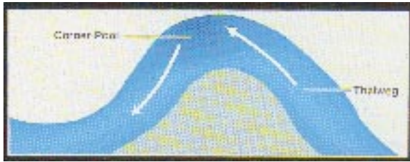
LATERAL SCOUR (LP) - CORNER
